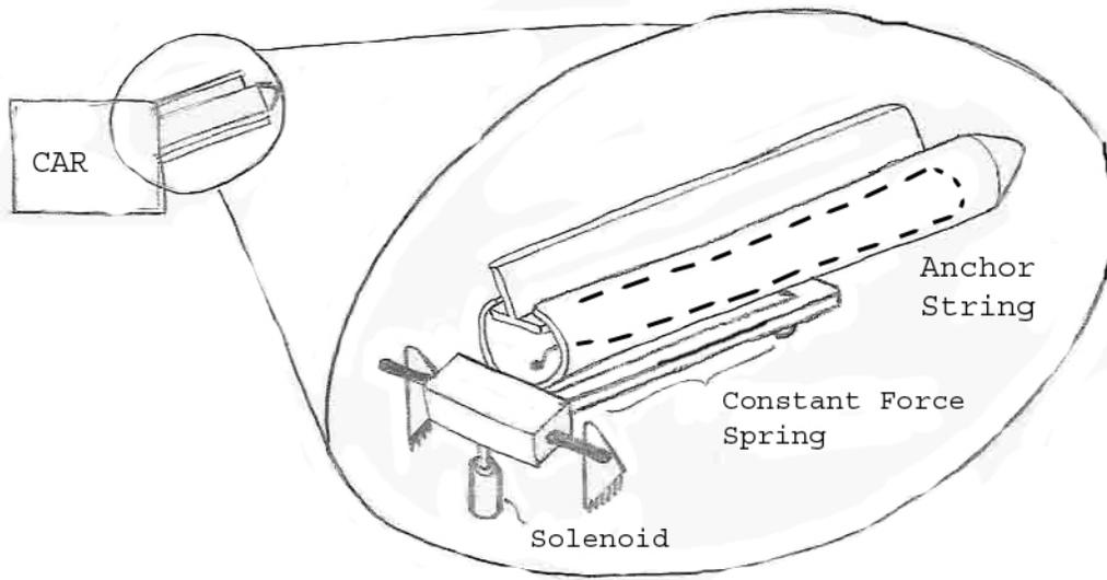
Figure 1: Projectile Mechanism
