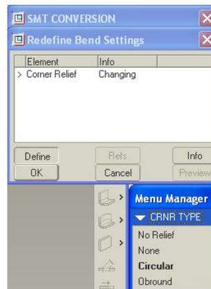
Accept by OK'ing boxes and **Done Sets**. This results in the Flat Pattern now showing large circular cut-outs at the corners. However, if the Flat Pattern is suppressed, it will be observed that the corners look the same as before on the folded-up version (ie with no relief). This is because the cuts cannot be computed until the fabrication is flat and, at the moment, the Flat Pattern feature is the first time that the sheet has been flat.
