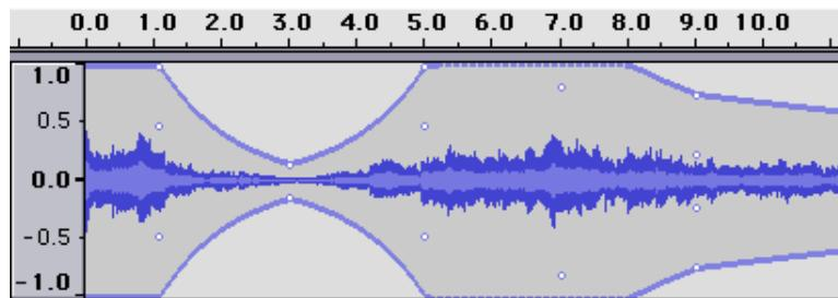
In the figure above, there are five control points, at 1.0, 3.0, 5.0, 7.0, and 9.0 seconds. Each control point has up to four "handles" arranged vertically. The top and bottom handles are positioned at the target volume, and the middle handles are positioned a quarter-screen down, giving you a way to move the envelope above the 1.0 level.
