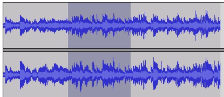
This is the waveform display part of the track, although it is also possible to display a spectrogram instead of a waveform here.
