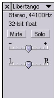
The track Control Panel appears directly to the left of every track. Clicking in the panel outside of one of its buttons or controls selects the entire track. Shift-clicking a track label adds or removes that track from the selection. Also, clicking and dragging a track label is one way to rearrange the order of tracks.
