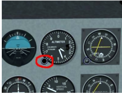
Figure 8.7: Altimeter calibration knob
