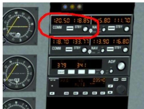
Figure 8.4: The C172 communications stack with COMM1 highlighted
