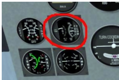
Figure 8.14: Fuel Flow and EGT gauges
