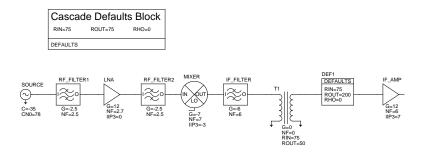
Figure 1: Simple Receiver Signal Chain Block Diagram
