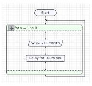
In this case we are using a for loop. The loop will execute until the value of x becomes nine. when x becomes greater than nine then loop will exit. Circuit is given below,
