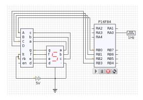
Practical cases replace the clock and include appropriate circuits, sample circuit below. The led light is cut the output will go high. We can use this circuit for counting number of persons entering the room etc.
