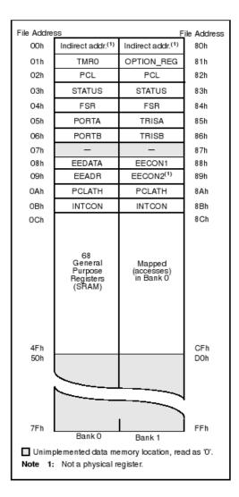
First thing you will notice is that it is split into two - Bank 0 and Bank 1. Bank 1 is used to control the actual operation of the PIC, for example to tell the PIC which bits of Port A are input and which are output. Bank 0 is used to manipulate the data. An example is as follows: Let us say we want to make one bit on Port A high. First we need to go to Bank 1 to set the particular bit, or pin, on Port A as an output. We then come back to Bank 0 and send a logic 1 (bit 1) to that pin.
