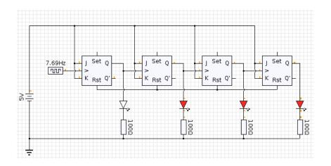
Note that there is a resitance connected between led and the output of the J-K flip flop(Q). This aviods the loading effect.
