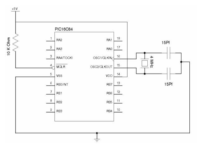
The above figure shows the basic circuit diagram of a PIC microcontroller (for any Pic series). A 4Mhz crystal is connected to the pin OSC 1 and OSC 2. MCLR is connected to the +5 volt supply through a 10 K Ohm resistance.
