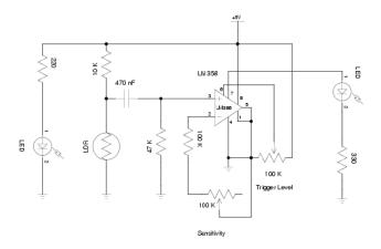
Components required IC LM 358, LDR, LED(red), Resistance(100k, 47k, 10k, 330 ohm and 220 ohm), preset(100k-2) and Capacitor(470 nF).
