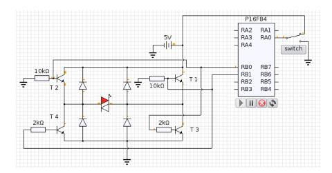
When RB0 is high transistor T2 and T3 conduct; current path is battery  $\rightarrow T2 \rightarrow motor \rightarrow T1$  and gound. when RB1 is high transistor T1 and T4 conducts; current path is battery  $\rightarrow T1 \rightarrow motor \rightarrow T4$  and gound. Doide's protect the transistor from back E.M.F
