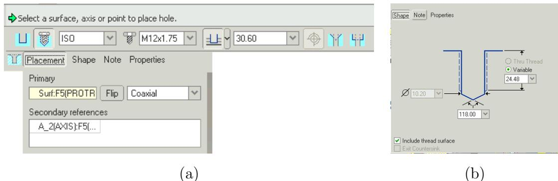
Figure 9: Hole dashboard. (a) Placement options & (b) Shape Options
