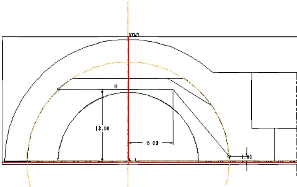
Figure 13: Dimensions of the large reinforcing rib
