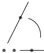
Figure 27: The Manual Intersection Snap tool also lets you specify invisible intersection points.
