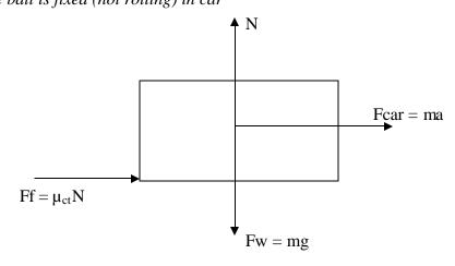
m = mass of car + mass of shot-put, a = acceleration of care,  $\mu_{ct}$  = friction coefficient between car and table
