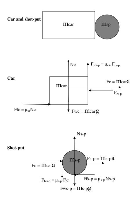
Frs-p = reaction force of the shot-put on the car,  $F_{fs-pc} = friction$  force between shot put and car
