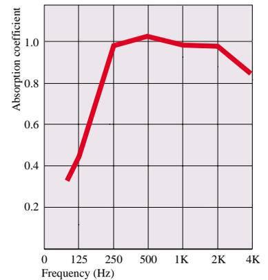
Rockwool Acoustic Element, standard size, fixed over a 50 mm cavity.
