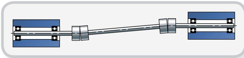
**Fig.19** Two single-stage couplings locate a fully-floating shaft on a stable axis of rotation.
