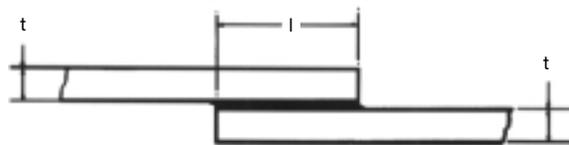
**Fig.12 Simple lap shear joint**
