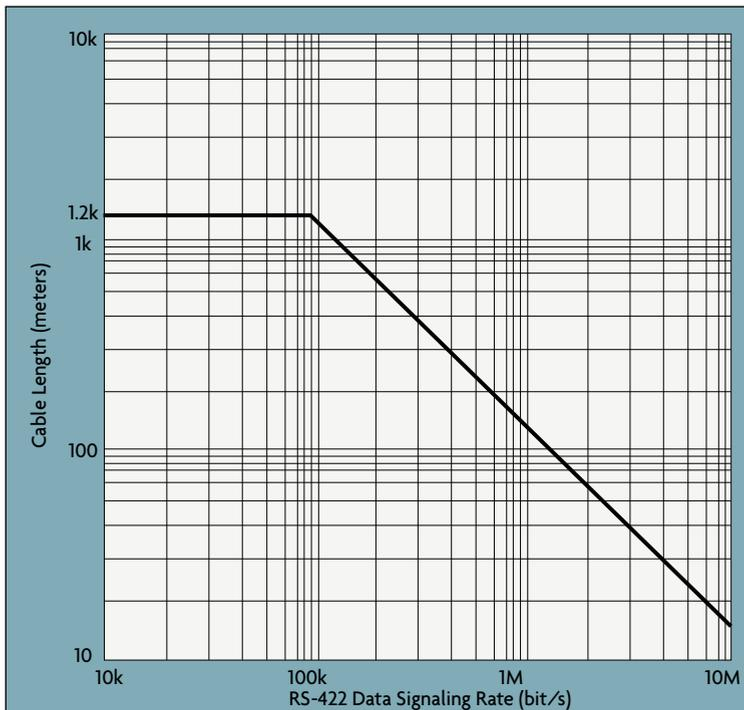
Figure 4-3: Cable Length vs. RS-422 Data Rate
