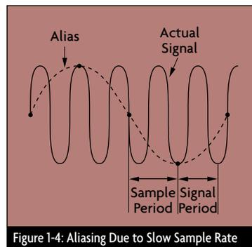
Figure 1-4: Aliasing Due to Slow Sample Rate
