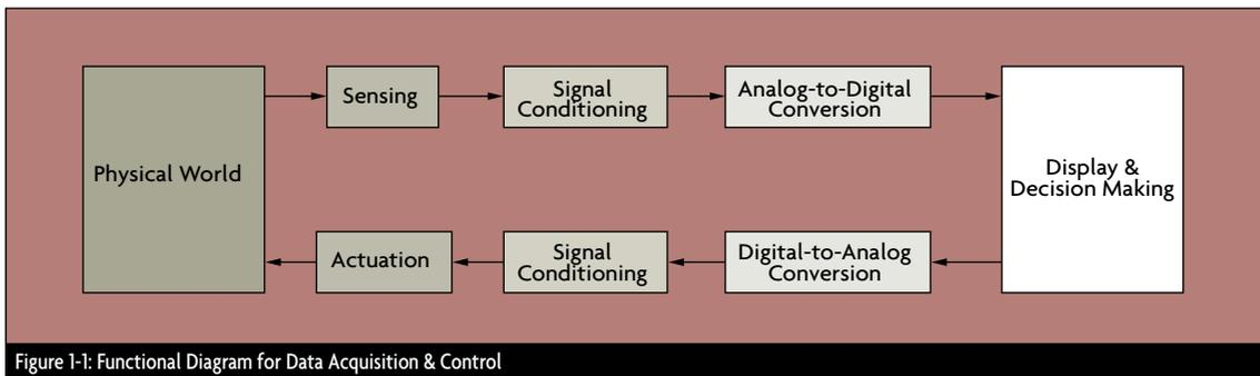
Figure 1-1: Functional Diagram for Data Acquisition & Control
