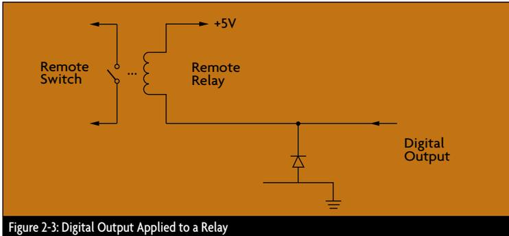
Figure 2-3: Digital Output Applied to a Relay
