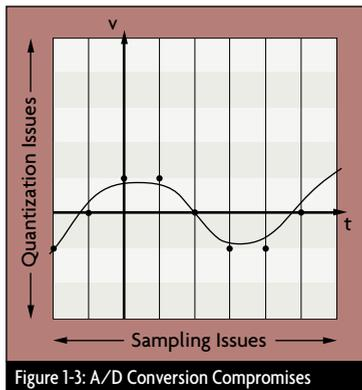
Digital data acquisition systems not only quantize data in terms of magnitude; time, too, is parceled into discrete intervals (Figure 1-3). In general, there is no information about the behavior of the process between data points gathered. Special precautions, then, must be taken to ensure no meaningful data is lost and interpolation between recorded points remains a valid assumption.
