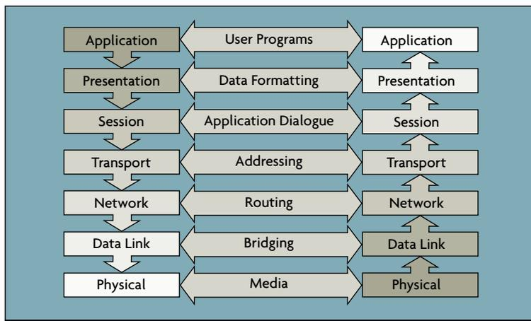
Figure 4-1: The Seven-Layer OSI Network Model
