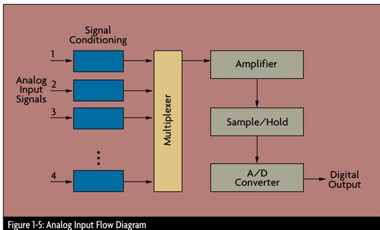
Figure 1-5: Analog Input Flow Diagram
