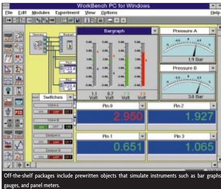
Off-the-shelf packages include prewritten objects that simulate instruments such as bar graphs, gauges, and panel meters.
