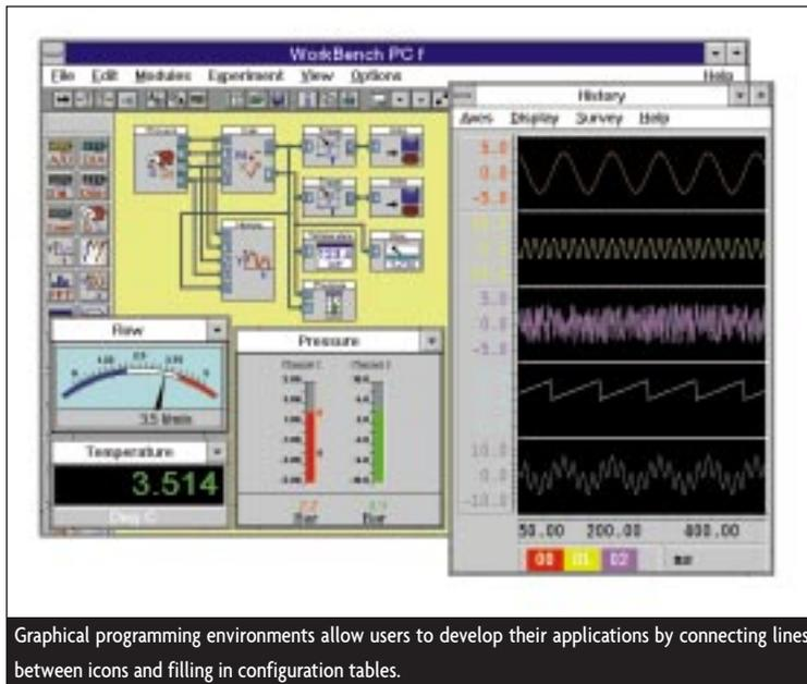
Graphical programming environments allow users to develop their applications by connecting lines between icons and filling in configuration tables.
