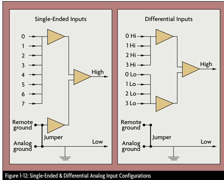
Figure 1-12: Single-Ended & Differential Analog Input Configurations
