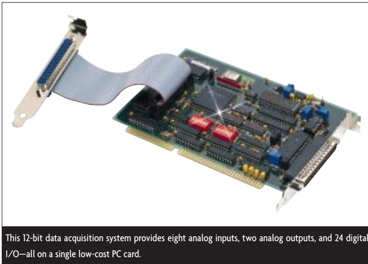
This 12-bit data acquisition system provides eight analog inputs, two analog outputs, and 24 digital I/O—all on a single low-cost PC card.
