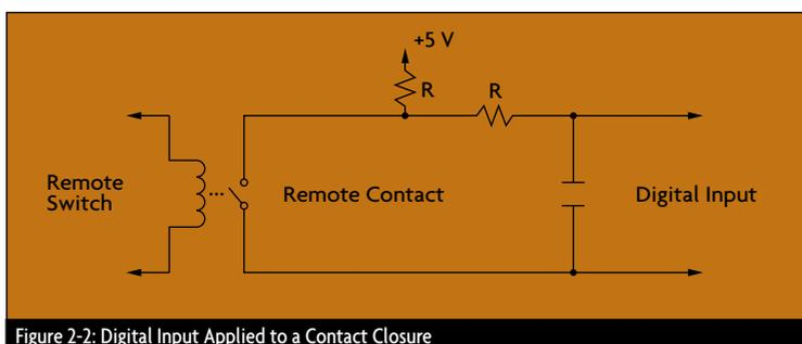
Figure 2-2: Digital Input Applied to a Contact Closure
