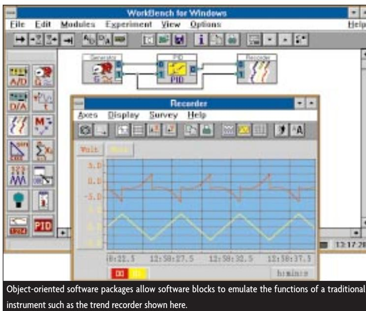
Object-oriented software packages allow software blocks to emulate the functions of a traditional instrument such as the trend recorder shown here.
