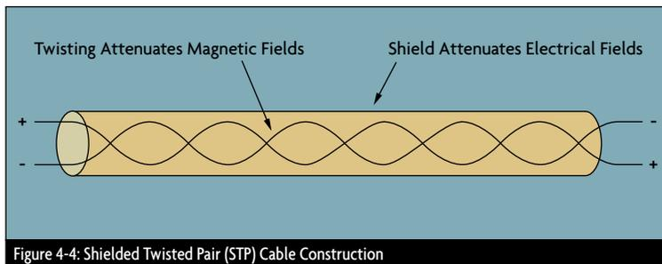
Figure 4-4: Shielded Twisted Pair (STP) Cable Construction
