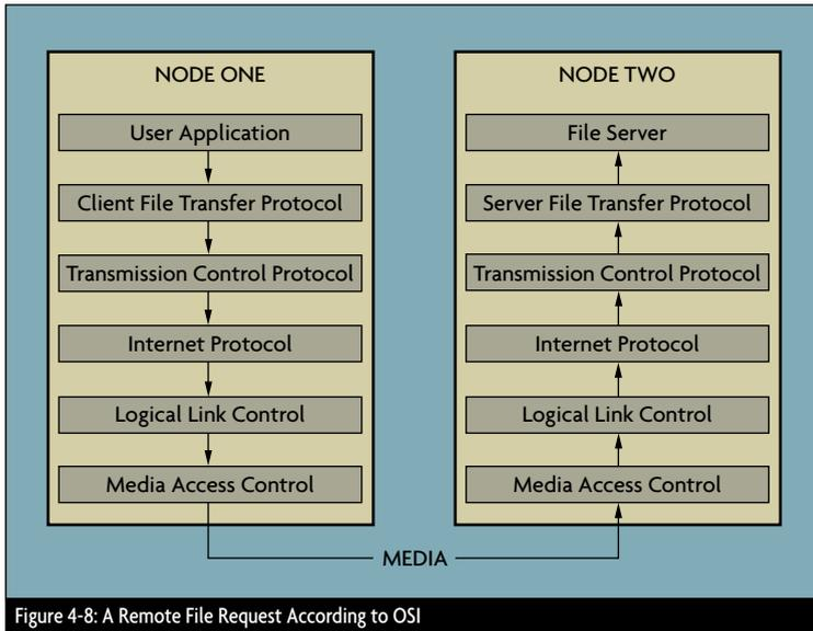
Figure 4-8: A Remote File Request According to OSI
